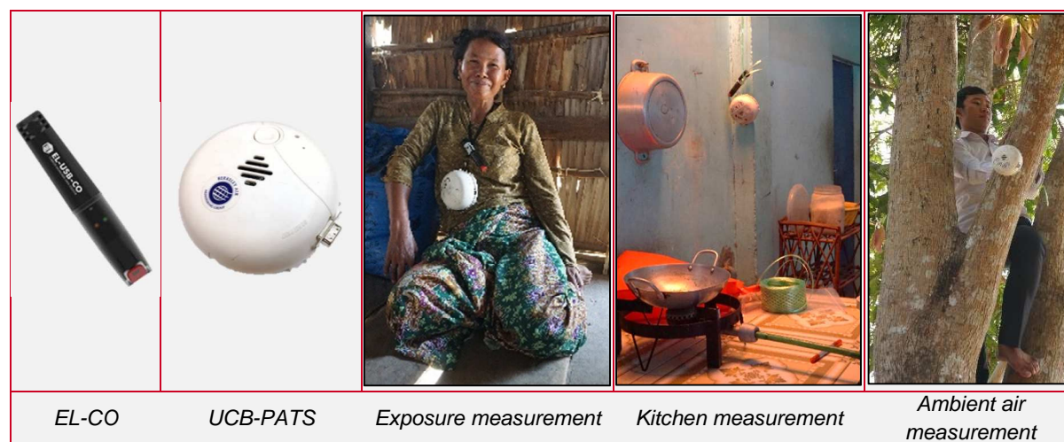
Figure 7: CO and PM2.5 data loggers and the measurement situations (main cook, kitchen and ambient)
